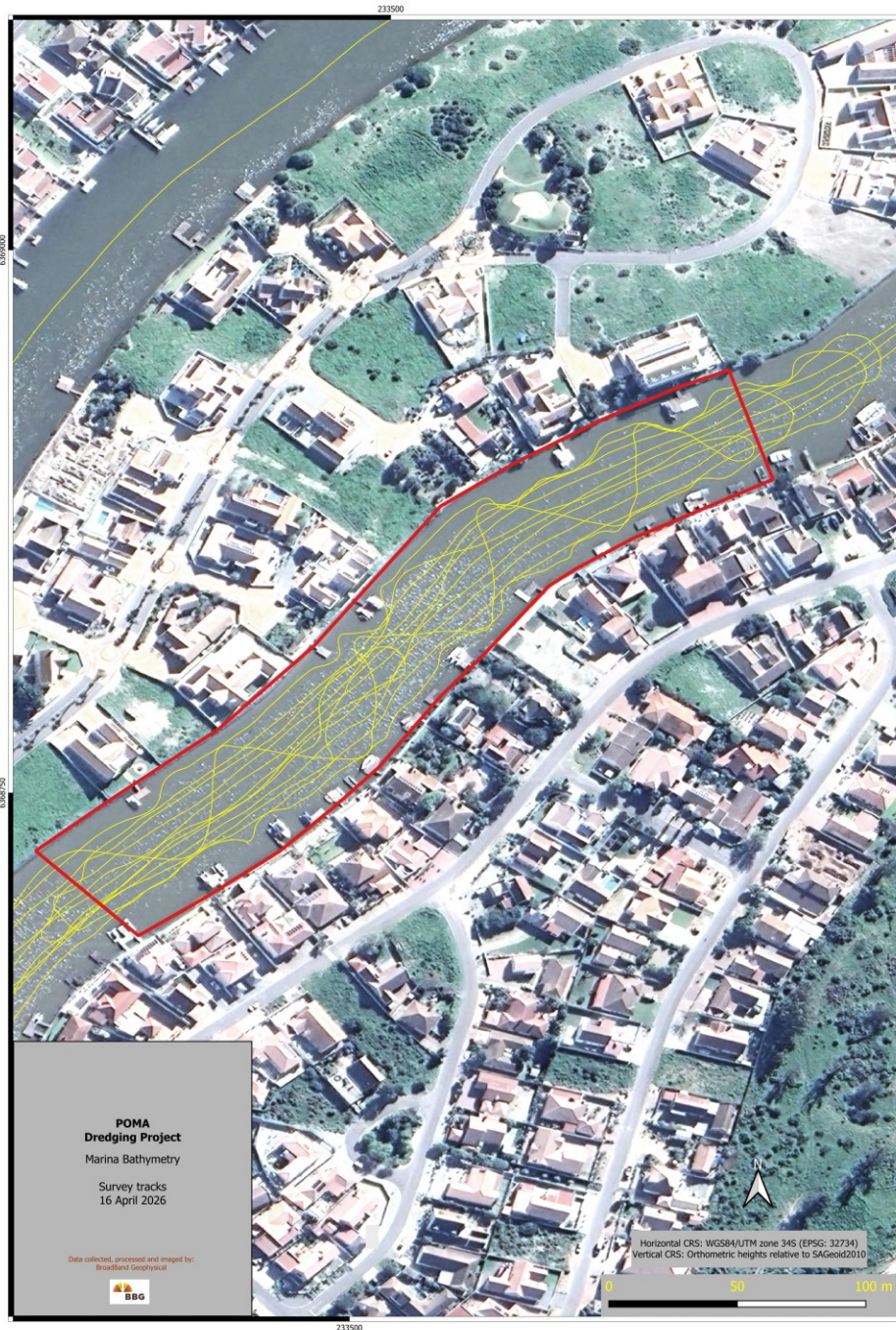
Figure 3 - Post-dredge Survey Tracks
