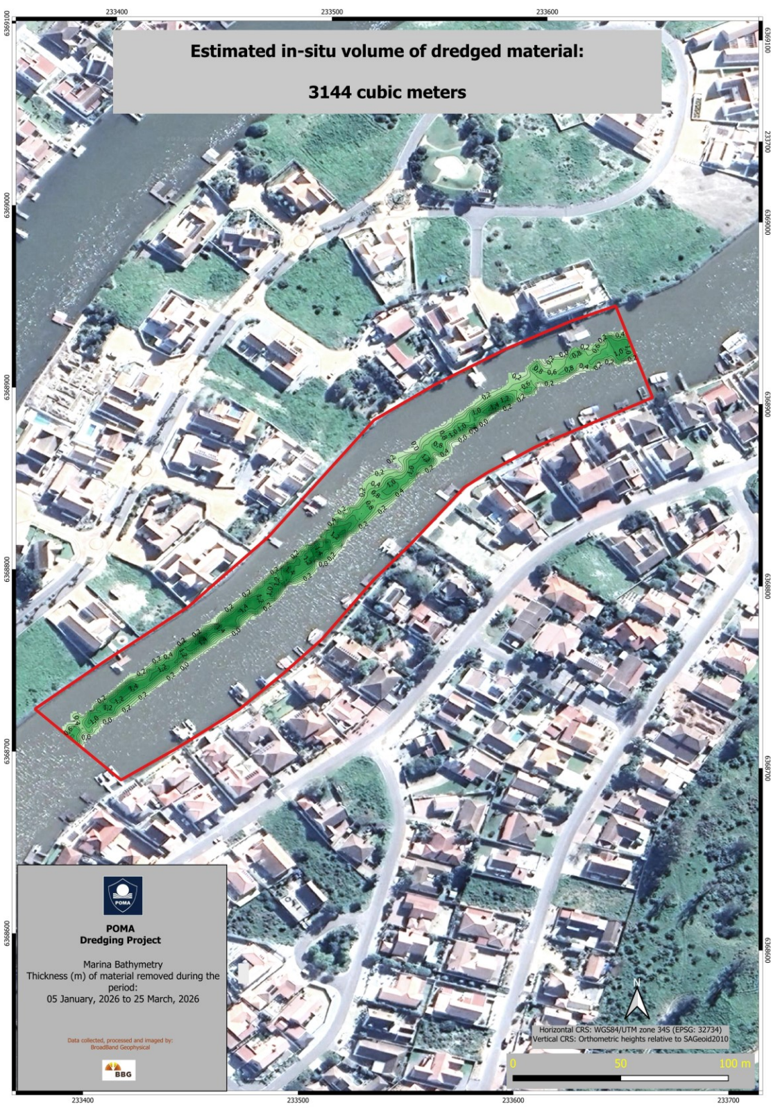
Figure 6 - Map showing in-situ thickness of material removed
